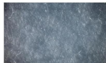
**Figure 4.** low angle light photos clearly show the pattern created by a state-of-the-art 2.5 layer traditional fabric (top) vs. a virtual mark-free sheet from an ESB fabric with plain weave surface and same sized MD/CMD yarns.
